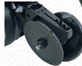
Cast iron "V" available as a repair part
