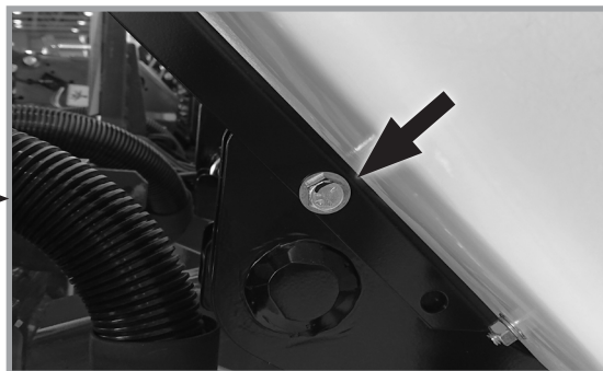
Undo and remove the cap screw
