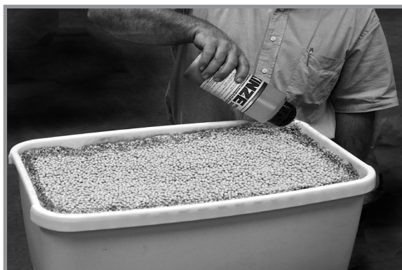
Adding graphite to conventional hopper
