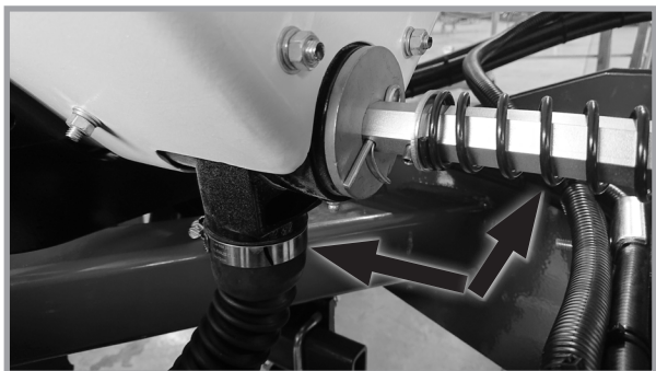
Disconnect drive shaft and hoses
