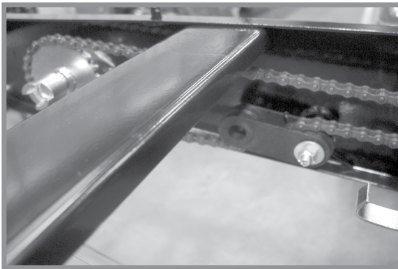
Row unit granular chemical drive
