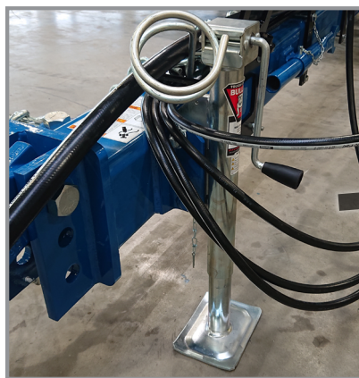
Jack stand installed
