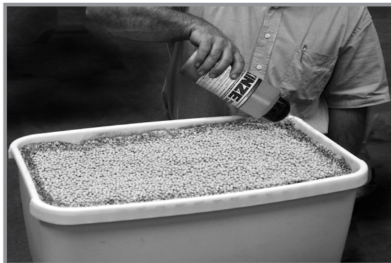
Adding graphite to conventional hopper
