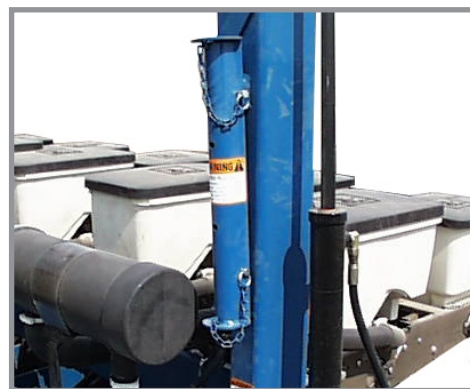
Row marker lockup in storage location
