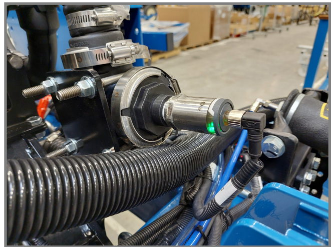
Sensor at the pump flow line
