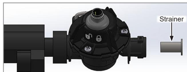
9. Reinstall gasket, orifice, and nozzle assembly.
