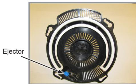
**NOTE:** Damaged seed or seed containing foreign material will cause plugging of seed disc orifices and require more frequent seed meter cleanout to prevent underplanting.
