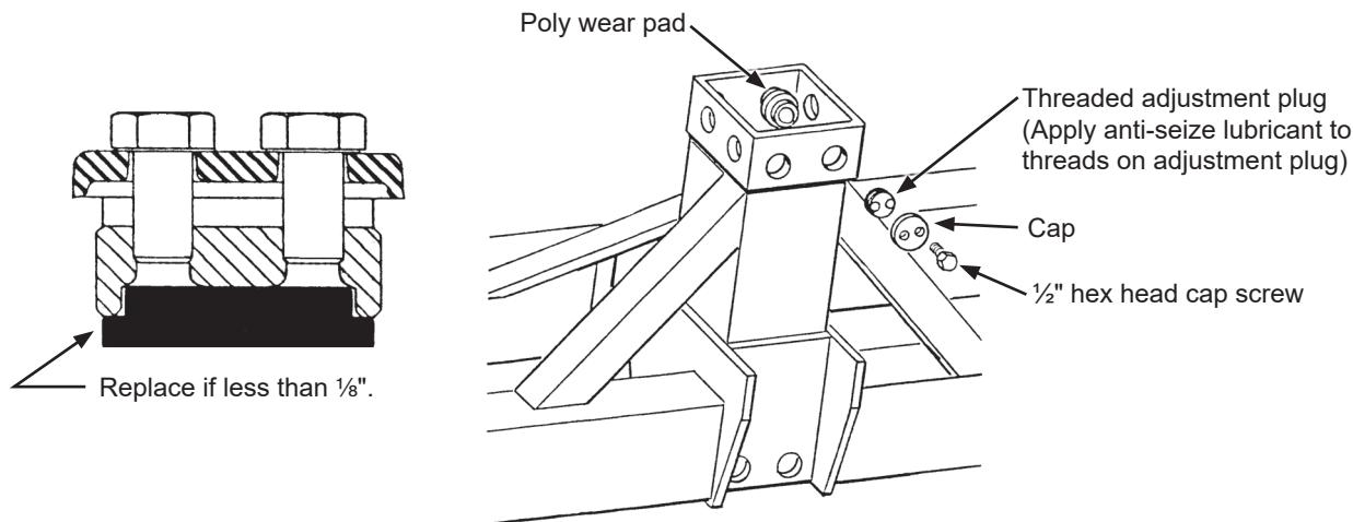
Planter center section consists of a steel tubular frame and 16 adjustable wear pad assemblies that travel up and down against a stainless steel clad center post. Each adjustable wear pad assembly consists of a poly wear pad, threaded adjustment plug, and cap. Assembly is held in place by the threaded adjustment plug and locked in place by the cap and two  $\frac{1}{2}$ " hex head cap screws.
