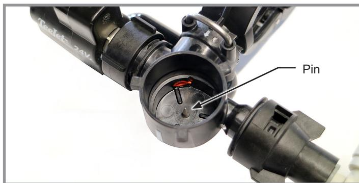
5. Reinstall cover and turn clockwise until the "lock symbol" is directly above the white line.
