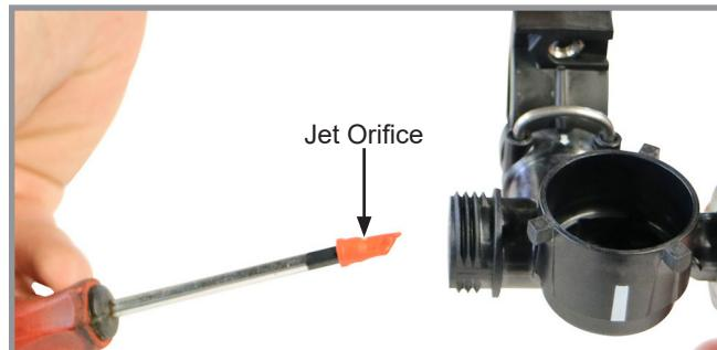
4. Insert jet orifice into center hole on the row shut valves, gently twisting back and forth to help align the rib on the orifice and the groove in the housing. The jet orifice should be flush with paddle wheel cavity wall when installed completely.
