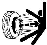
Explosive separation of rim and tire parts can cause death or serious injury. Overinflation, rim and tire servicing, improper use of rims and tires, or worn or improperly maintained tires could result in a tire explosion.
