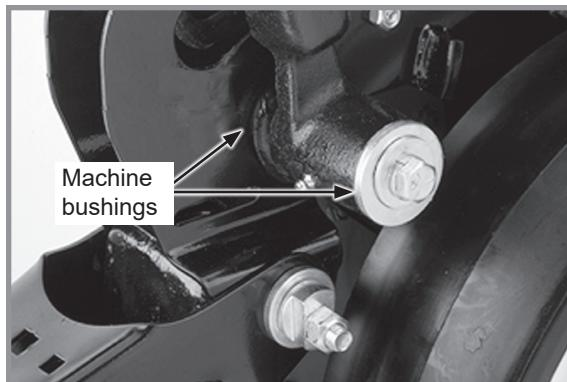
**NOTE: It may be desirable to space gauge wheel further from blade when operating in sticky soils.**
