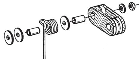
NOTE: Reverse idler when worn on one side for extended use.
