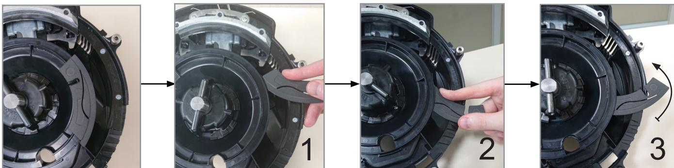
1. Begin inserting the Insulation Shim by sliding the tail end of it inside the gap indicated above, knife-like (img. 1).
