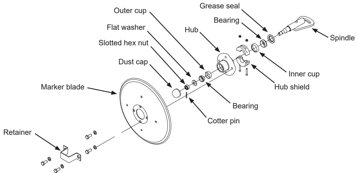
1. Remove retainer and marker blade.
