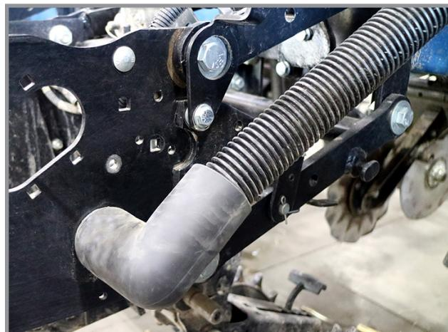
When push row units are not used, move row unit end of 2" (5 cm) vacuum hose on each push row unit to storage mount located on side of shank.
