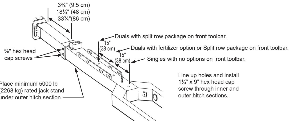
1. Lower machine to field position and block transport wheels.
