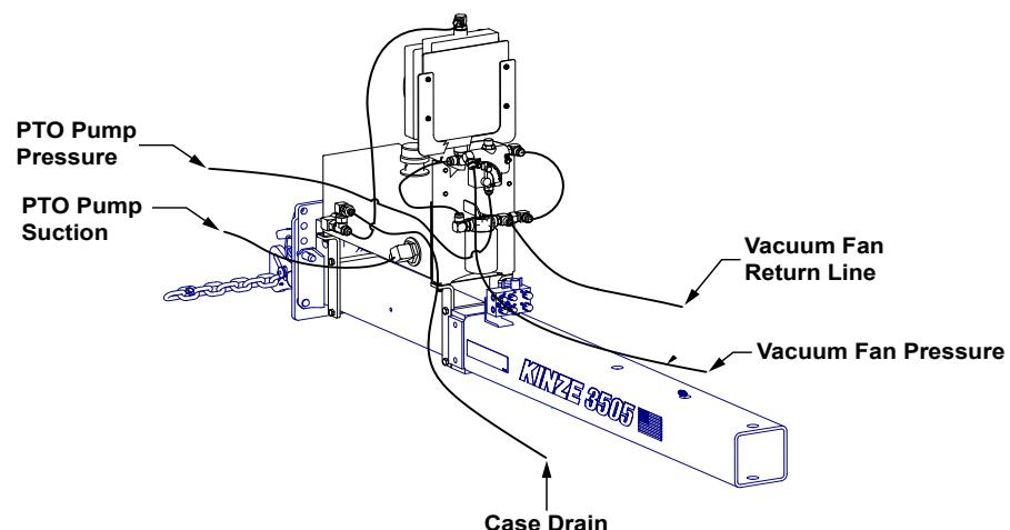
**BLUE DRIVE BLUE VANTAGE PTO PUMP DRIVE AND OIL COOLER OPTION****Vacuum/Conventional**
