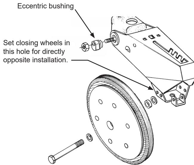
“V” Closing wheels installed offset
