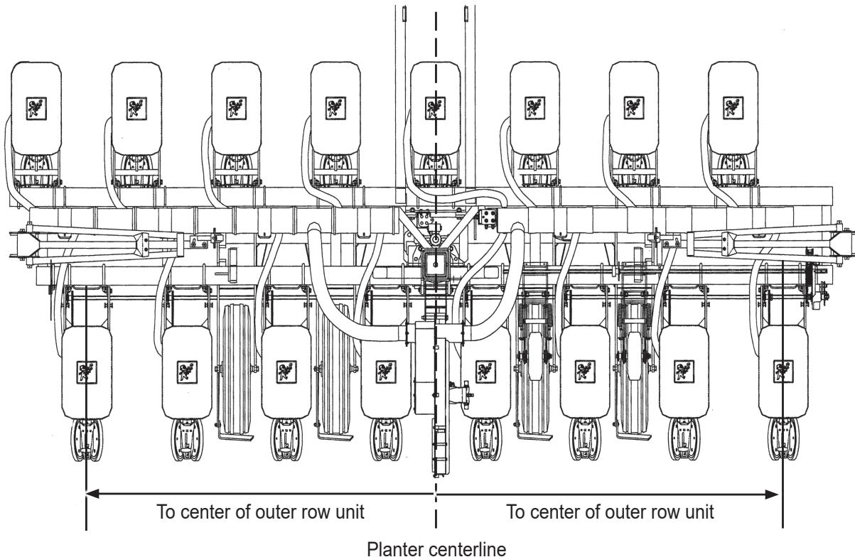
Center of planter to center of outer row unit.  $x 2 + 35 \text{ cm} = \text{Dimension between planter center line and marker blade}$
