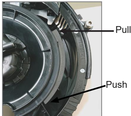
To remove the Insulation Shim, push down with your fingers on one end, while pulling on another end (see img. above).
