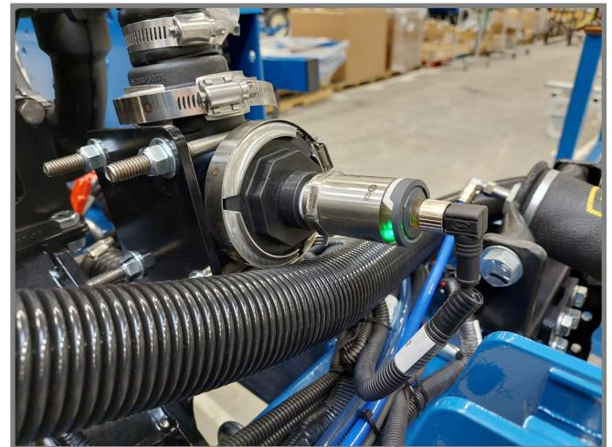
Sensor at the pump flow line
