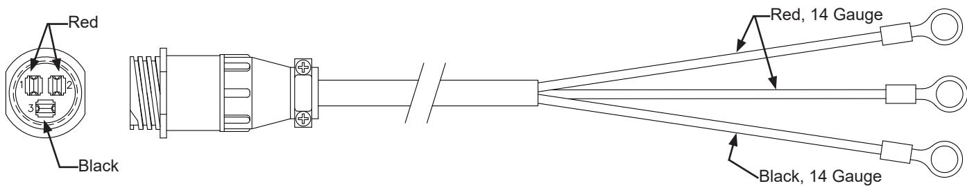
**PDP Display Harness (Ground Contact Drive)**
