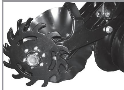
Residue wheels attach to row unit mounted coulter with two cap screws and sleeves allowing unit to free-float. A 2-position spindle bolt mounting positions wheels interlocked or staggered. Depth adjustment is made with a spring-loaded cam and pin with 11 positions in  $\frac{1}{4}$ " (~6 mm) increments. A high point on the cam allows wheels to be locked up.
