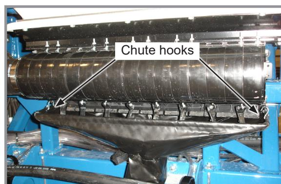
Cleanout chute installed
