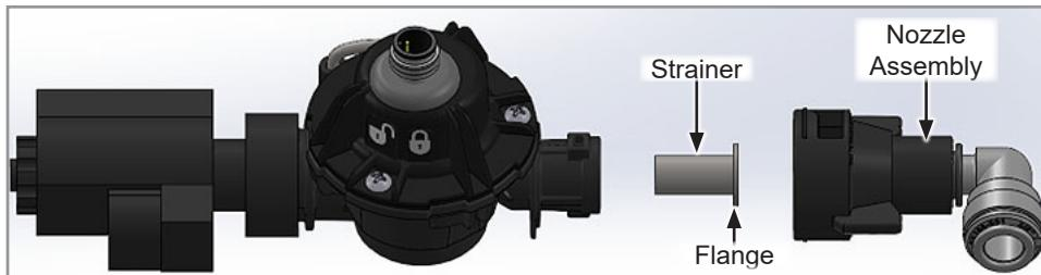
2. Pull strainer out of flow meter and clean or replace it.
