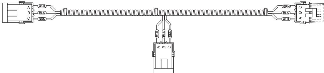
**Cable Power Adapter (Ground Contact Drive)**
