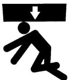
Falling equipment can cause death or serious injury. Install all lockup devices or lower planter to ground before working on equipment.
