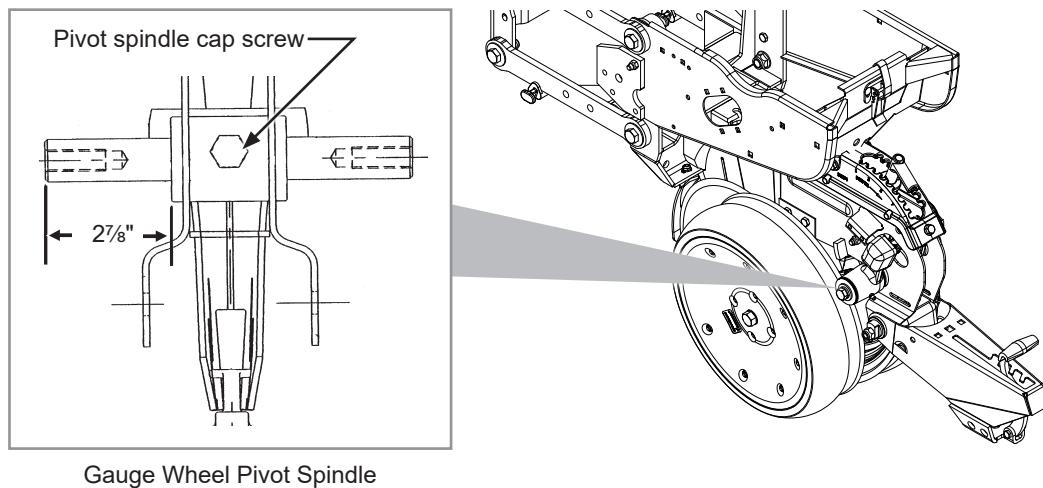
1. Remove gauge wheel and arm assemblies from shank assembly.
