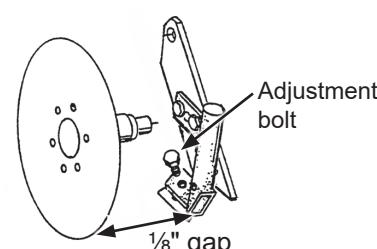
Adjust liquid drop tube/scraper so there is slight contact between blade and scraper lower leading edge, and  $\frac{1}{4}$ " (0.6 cm) clearance between liquid drop tube trailing edge and blade. Blade should turn with minimum amount of drag.
