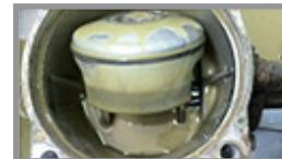
Oil After Diaphragm Rupture
