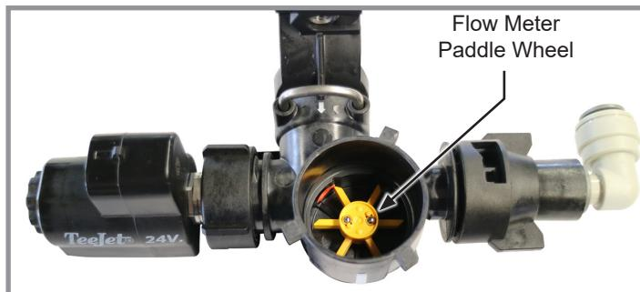
3. Rotate the nozzle assembly counterclockwise 90° and pull nozzle off.
