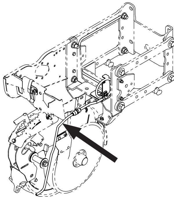
In Furrow is available for in-line installation to ensure equal distribution of product at low rates and siphon protection for field turns.
