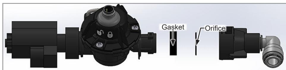
**NOTE: Orifices must be installed correctly. Install orifice with the blank side towards the flow meter manifold and the stamped side facing nozzle assembly (pointing downstream toward the direction of delivery).**
