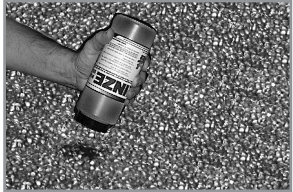
Adding graphite bulk fill hopper
