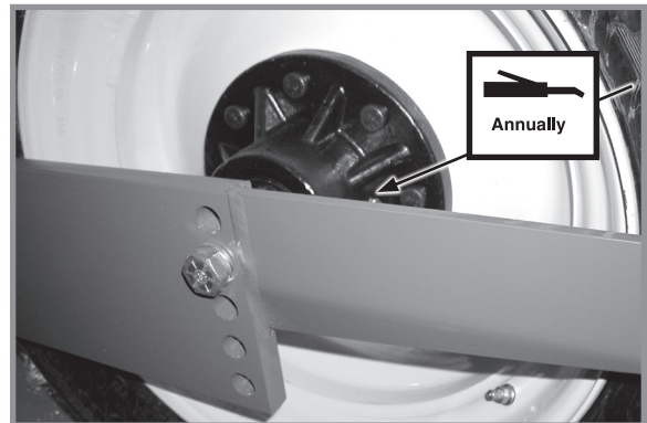
Transport wheel bearings - 1 per hub
