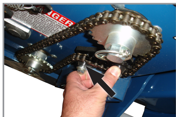
Chain idler tensioning
