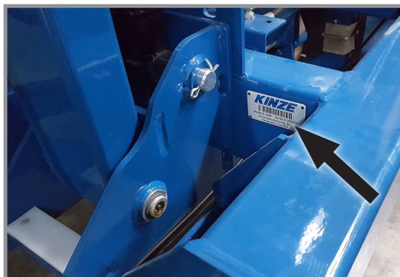
Serial number plate location - Outer R.H. Wing (2021 Production And On)
