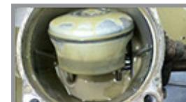
Oil After Diaphragm Rupture
