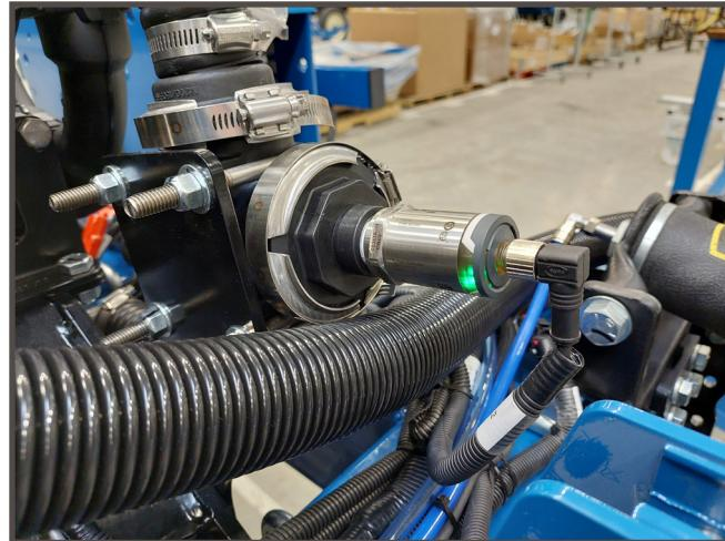
Sensor at the pump flow line
