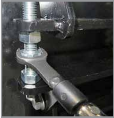
Torque Turnbuckles hardware to 5 ft-lbs
