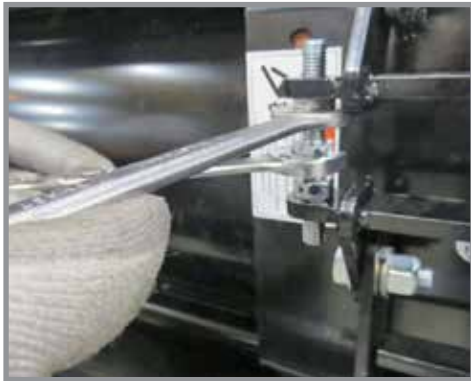
Hold turnbuckle in place, tighten both top and bottom jam nuts.
