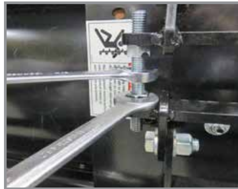
Hold turnbuckle in place, tighten both top and bottom jam nuts.
