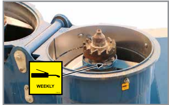
Vertical Auger Center Bearing - 1 Zerk (2022 Production)
