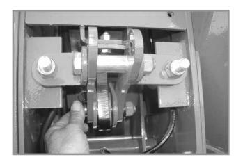
The V-belts are tensioned by a spring-loaded idler. Two springs are used to maintain even pressure across the V-belts. Set spring tension at 23/4" as shown below.
