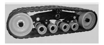
2. Remove five mounting bolts, remove top roller wheel, and then remove hub cover.
