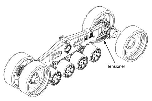
The tensioning system is located between the 2 rear idlers. The tension force is provided by a mechanical spring mechanism. Track tension is provided by the spring and does not need adjustment during operating and changing field conditions. Provisions are made to compress the spring allowing for removal of idlers and track assemblies during maintenance and servicing. Special tools are available from Kinze to compress the spring and detension the tracks.
