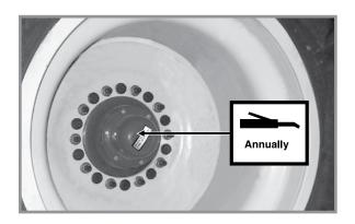
Horizontal Auger Idler Pivot - 1 Zerk
