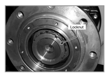
6. Align one of four lock nut slots in the lock nut with nearest tab on locking washer. Bend lock washer tab into slot.
