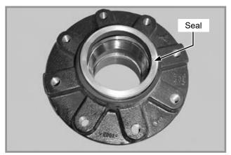
2. Flood collar ring with denatured alcohol to remove any dust or lint from seal cup. Use installation tool to install face seal assembly on collar ring. Install inner bearing cone on axle.
