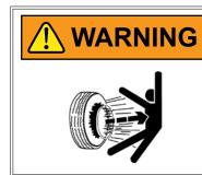
Explosive separation of rim and tire parts can cause death or serious injury. Overinflation, rim and tire servicing, improper use of rims and tires, or worn or improperly maintained tires could result in a tire explosion.
