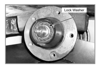
4. Remove thrust washer, remove outer bearing, and remove hub.
