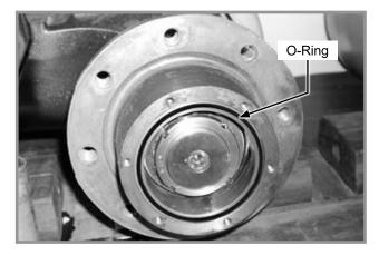
8. Install hub cover and six retaining bolts. Tighten bolts in a cross pattern evenly to 132 in-lb (11 ft-lb) (15 Nm).
