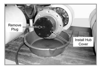
9. Remove plug and fill hub with 7.3 fl oz (215 ml) of Northland Transdraulic Fluid or equivalent. Oil level must be at bottom of fill plug hole. Tighten plug to 25 ft-lb (34 Nm).
