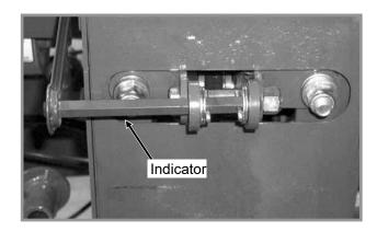
6. Loosen two carriage bolts on belt slide to gain clearance for belt removal.
