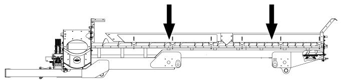
Factory-installed restrictor plates can be adjusted to control volume of grain to the horizontal auger.
