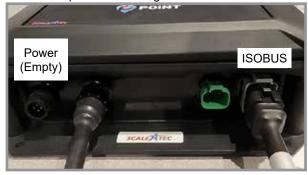
Check the other end of the Scale-Tec ISO harness. The 9-pin port on the back of tractors is often dirty and the connector may not have a good retaining mechanism.
