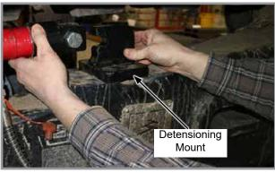
NOTE: Ensure Porta Power hose is positioned as shown to avoid interference when removing idler wheel.
