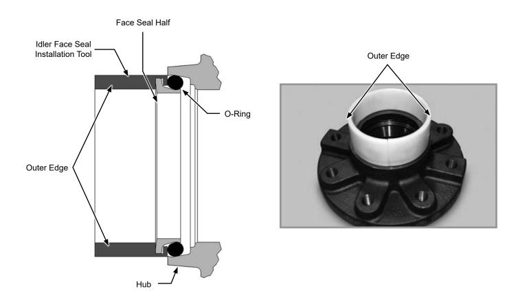
1. Lubricate seal load ring with denatured alcohol use the service installation tool to install seal and load ring in hub.
