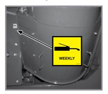
Vertical Auger Center Bearing - 1 Zerk (2022 Production)
