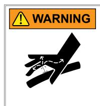
Pressurized hydraulic fluid can penetrate body tissue and result in death, serious infection, or other injuries. Fluid injected under skin must be IMMEDIATELY removed by a surgeon familiar with this type of injury. Make sure connections are tight and hoses and fittings are not damaged before applying system pressure. Leaks can be invisible. Keep away from suspected leaks. Relieve pressure before searching for leaks or performing any system maintenance.
