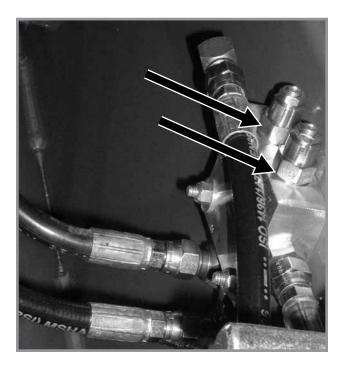
Counter balance valves prevent the auger fold cylinder from extending or retracting without applied hydraulic pressure. If the valve(s) fail to lock the auger in position or fail to function properly, remove the valve(s) from the valve block and check for foreign material. Replace valve if found to be defective.
