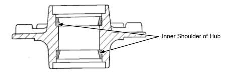
2. Use denatured alcohol to clean inner bearing cup and seal contact area. Wipe seal contact area with a clean lint free cloth.
