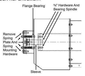
Position the vertical auger in a horizontal position as illustrated.
