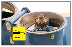
Grease Bank (Auger Bearings and Linkages) - 1 Zerk Each
