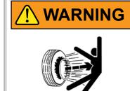
Over-inflation of tires can result in explosive separation of rim and tire and cause death or serious injury. Different size rims are designed for different tire pressures. Inflate to correct pressure for specific rim size.
