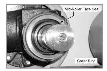
4. Remove outer face seal and load ring from hub.
