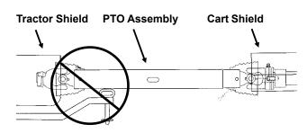
2. Connect auger cart to tractor hitch. Irregardless of hitch option (bolt-on single clevis, bolt-on double clevis or swivel single clevis), use a high quality hitch pin of sufficient length and strength and secure pin with a locking device.
