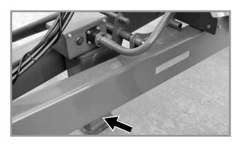
5. Position jack handle as shown below. Use the jack handle to rotate the jack enough to allow removal of the L-pin.
