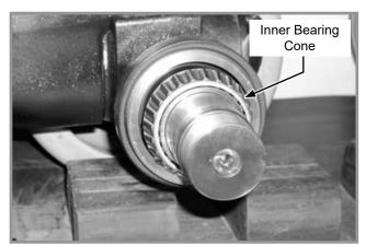
Carefully install hub assembly on axle without dislodging inner bearing and face seal until face seals make contact. Hold hub assembly in Steps 4 and 5.
