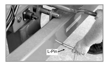
6. Rotate parking jack to the horizontal storage position to prevent damage to jack in uneven operating conditions. Install L-pin to lock the jack in the raised position. Return jack handle to storage location.
