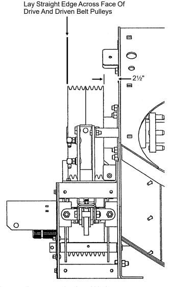
NOTE: Pulleys do not need to be loosened to remove/replace V-belts.
