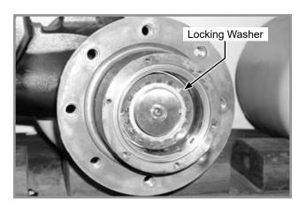
Install locknut and tighen to 32 ft-lb (43 N-m).
