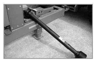
NOTE: The PTO must remain disconnected and positioned as far to the right of the cart hitch as possible until the parking jack is raised.
