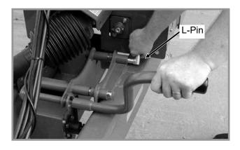
7. Attach cart PTO connecting yoke to tractor PTO shaft. Be sure spring loaded yoke pin engages groove in tractor PTO shaft. Check that slip tube grease fitting is visible through hole of outer tube.
