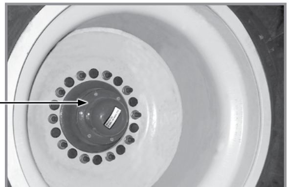
Flotation Carts (20 Bolt Hub) Wheel Bearings (Qty. 1 Per Wheel Hub)
