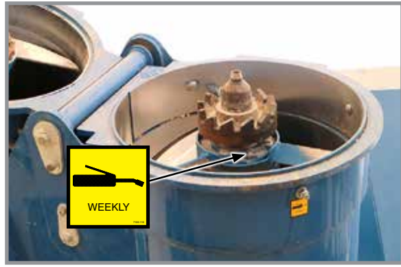
6. Grease Bank (Auger Bearings) - 1 Zerk Each (2023 Production and On)
