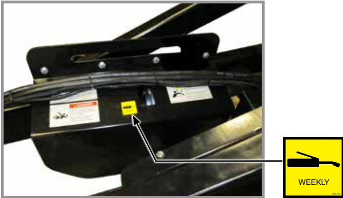
3. Cam Rollers - 1 Zerk (2022 Production)
