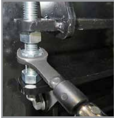
Torque Turnbuckles hardware to 5 ft-lbs
