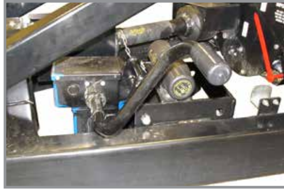
Jack handle installed
