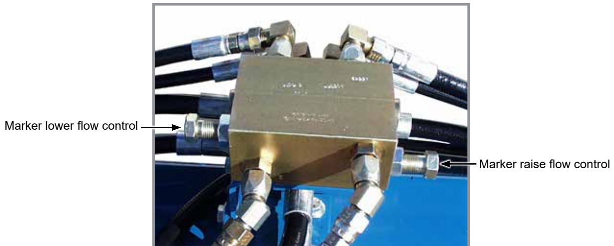
Row marker flow control valves
