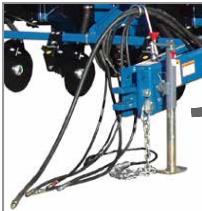
Jack stand installed
