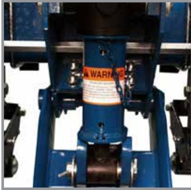
Safety lockup installed
