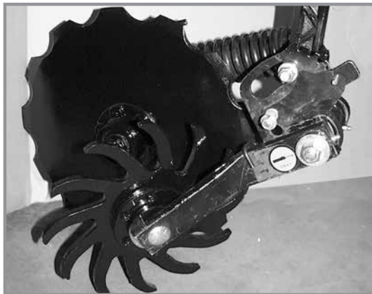
Notched single disc opener residue wheel attachment
