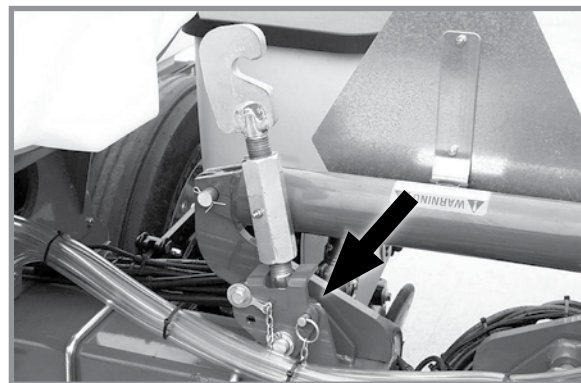
Center turnbuckle lockup pin
