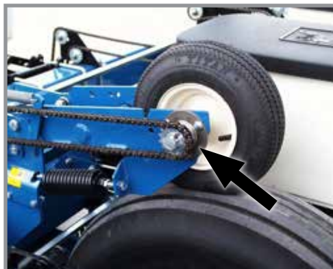
Contact wheel drive sprocket
