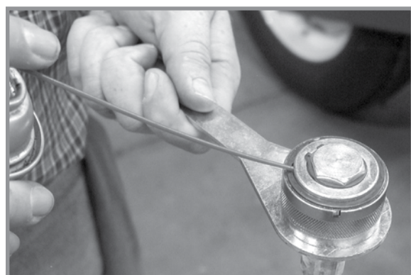
Wrap Spring Wrench Lubrication
