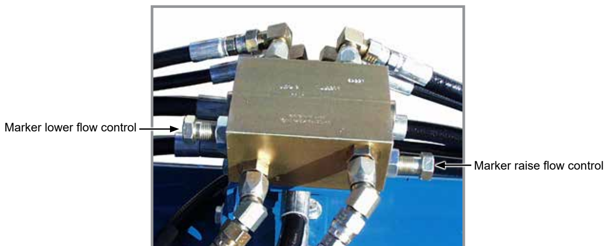
Row marker flow control valves
