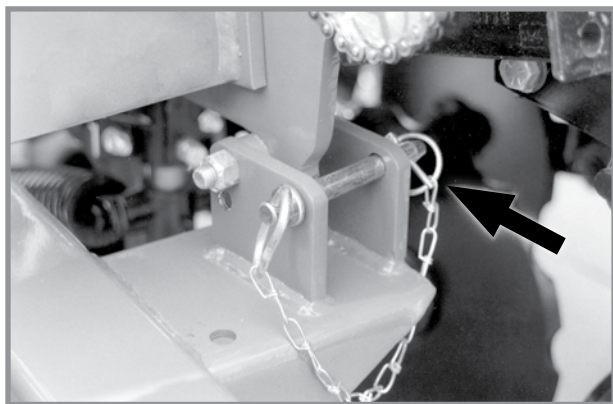
Wing safety pin in transport position
