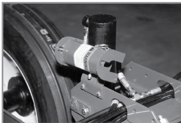
Lift cylinder lockup in storage position
