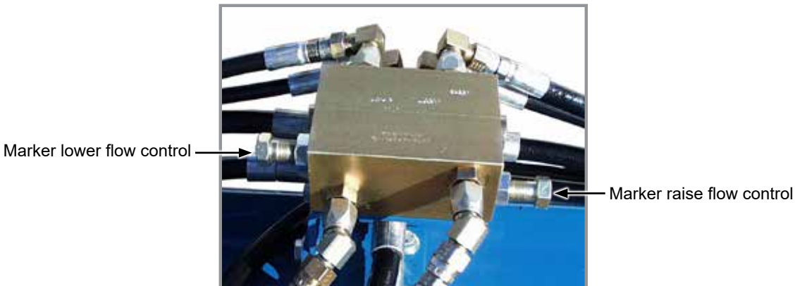
Row marker flow control valves
