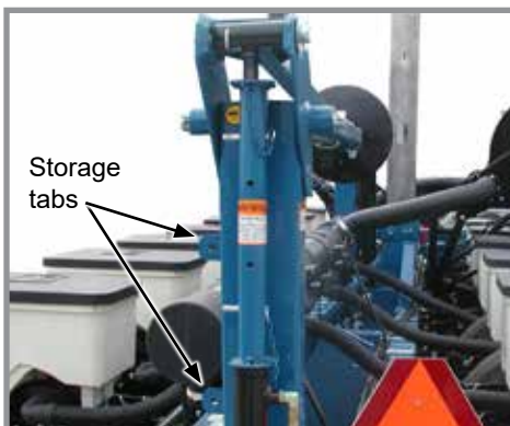
Row marker lockup installed
