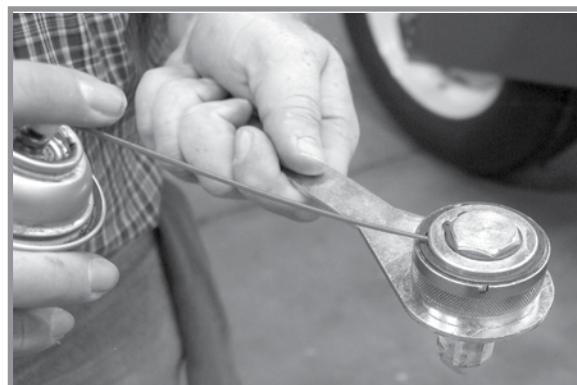
Wrap spring wrench lubrication
