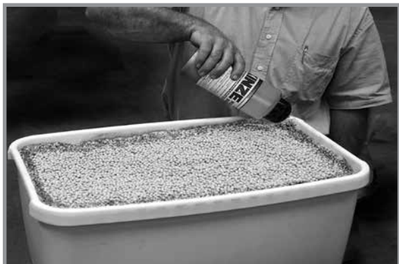
Adding graphite to conventional hopper
