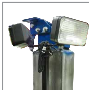
Auxiliary work lights
