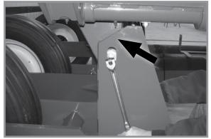
Adjust and tighten cam roller
