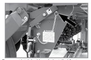
Transport latch locking pin installed for transport
