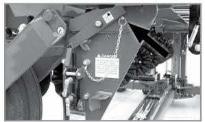
Transport latch locking pin installed
