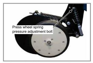
Press wheel down pressure adjustment
