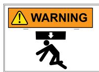
Uncontrolled movement of equipment can cause loss of control and could result in death, serious injury, or damage to property and equipment. Install all safety pins before transporting equipment.
