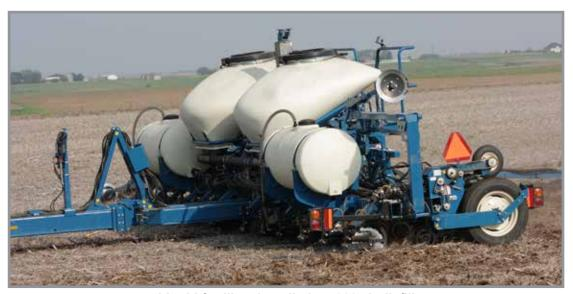
Liquid fertilizer installed on 3605 bulk fill
