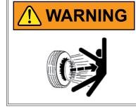
Over-inflation of tires can result in explosive separation of rim and tire and cause death or serious injury. Different size rims are designed for different tire pressures. Inflate to correct pressure for specific rim size.
