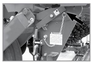
Transport latch locking pin Locked transport position
