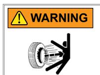
Loose transport wheel lug bolts can result in wheel separation from planter and result in death, serious injury, and damage to property and equipment. Check transport wheel lug nut torque before operating planter for the first time and periodically thereafter.
