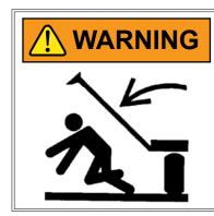
Row marker can lower at any time and could cause death or serious injury. Stay away from row markers! Install safety lockup device when not in use.
