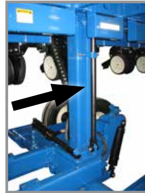
Safety lockup in transport/maintenance position
