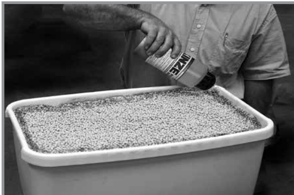
Adding graphite to conventional hopper
