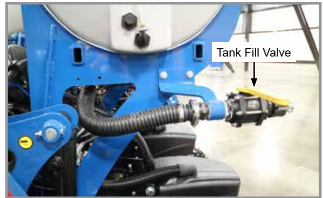
150 Gallon Liquid Fertilizer Tank Fill Location
