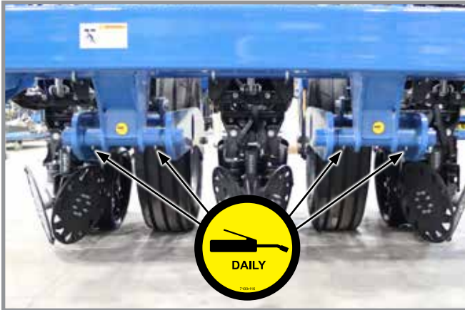
7. Wheel Modules 4 fittings per wing wheel 4 wing wheels (16 Row); 2 wing wheels (12 Row)
