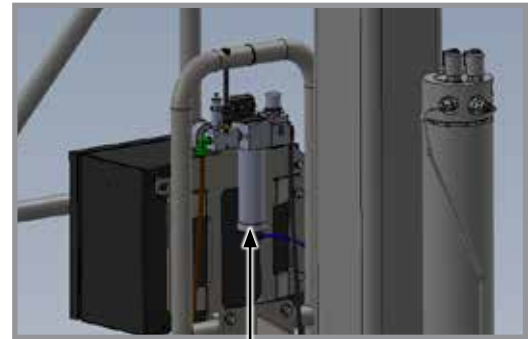
Air to Water Separator
