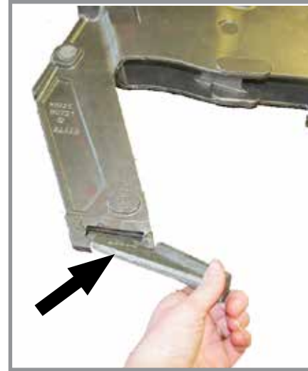
Seed Tube Guard/Inner Scraper (Gauge wheel/seed opener disc blade removed for easier identification of scraper) True Rate Scraper Shown
