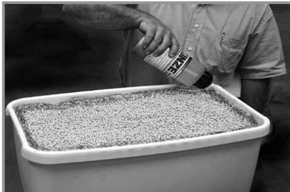
Adding graphite to conventional hopper
