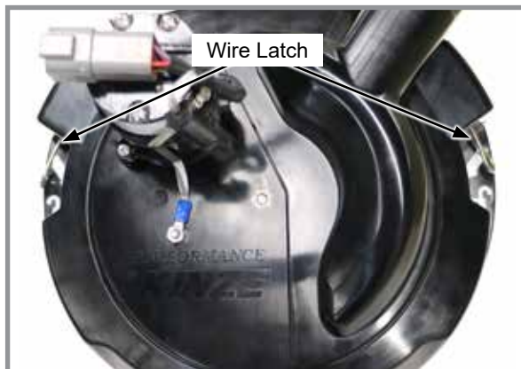
Style B: Push wire latch down on each side of cover to unlock, pull towards you to rotate out and remove.
