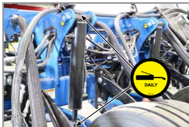
8. Wing lift cylinders 2 fittings per cylinder 4 cylinders (16 Row); 2 cylinders (12 Rows)
