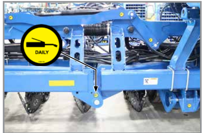
2. Wing hinges 2 fittings per hinge - 2 hinges
