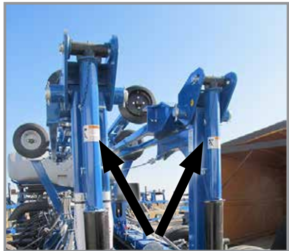
Row Marker Safety Lockup Installed
