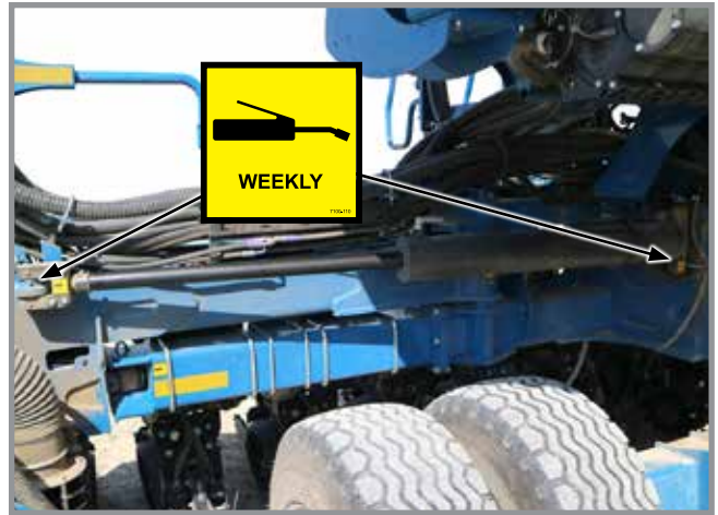
2. Wing Fold cylinders, 4 per machine 2 fittings per cylinder (one each end)
