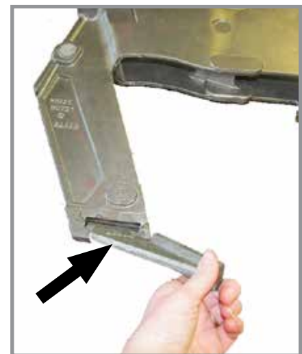
Seed Tube Guard/Inner Scraper (Gauge wheel/seed opener disc blade removed for easier identification of scraper) True Rate Scraper Shown
