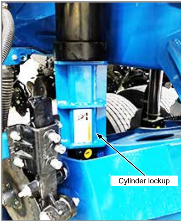
Transport axle cylinder lockup installed
