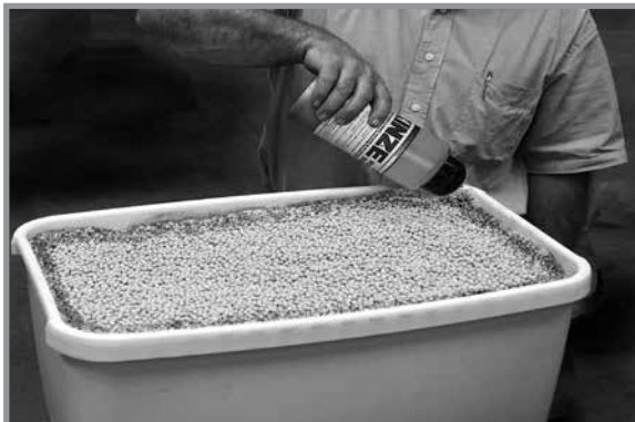
Adding graphite to conventional hopper
