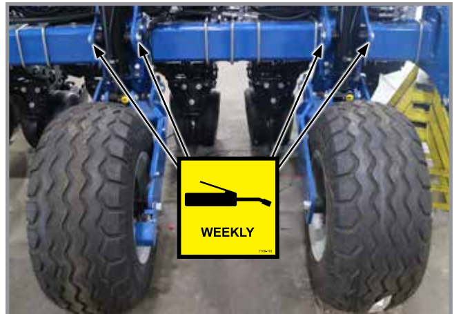
5. Lift Cylinders, 12 per machine 3 fittings per cylinder
