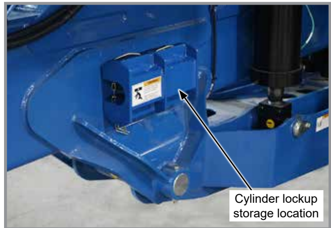
Cylinder lockup storage location
