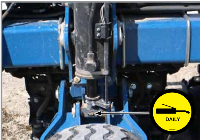
5. Lift Cylinders, 12 per machine 3 fittings per cylinder
