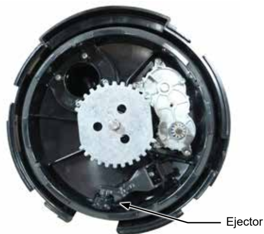
Seed Meter With Back Cover Removed
