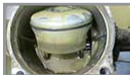
Oil After Diaphragm Rupture
