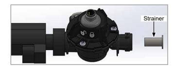
9. Reinstall gasket, orifice, and nozzle assembly.
