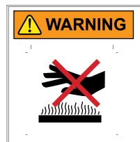
Serious burn injuries could occur from touching exposed metal parts such as compressor head, copper/braided discharge lines, and hydraulic motor during operation and even after compressor is shut down for sometime.
