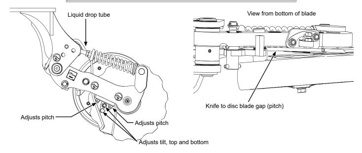
Check knife to disc blade clearance and adjust if necessary as described below.
