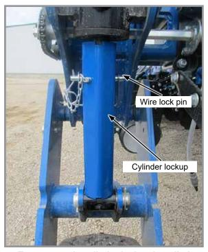
Transport axle cylinder lockup installed
