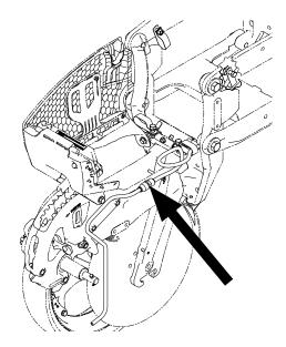
In Furrow is available for in-line installation to ensure equal distribution of product at low rates and siphon protection for field turns.
