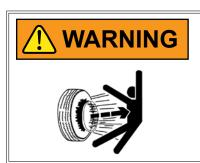
Loose transport wheel lug bolts can result in wheel separation from planter and result in death, serious injury, and damage to property and equipment. Check transport wheel lug nut torque before operating planter for the first time and periodically thereafter.
