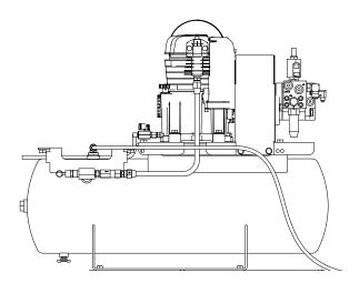
Prior to daily operation check the oil in the compressor when the planter is on level ground. The oil level can be checked in the clear sight glass on the end of the compressor. Always maintain oil level to read 2/3 full on the sight glass. Oil levels over this amount can result in oil blowing past rings or through crankcase breather. Lower amounts of oil can result in insufficient lubrication of moving parts.
