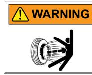
Overinflation of tires can result in explosive separation of rim and tire and cause death or serious injury. Different size rims are designed for different tire pressures. Inflate to correct pressure for specific rim size.
