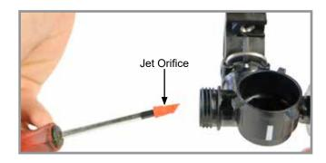
4. Insert jet orifice into center hole on the row shut off valves, gently twisting back and forth to help align the rib on the orifice and the groove in the housing. The jet orifice should be flush with paddle wheel cavity wall when installed completely.
