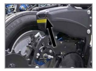
Use the manual run button to turn on the seed meter and all optional equipment on each row unit to check functionality.
