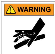
Pressurized hydraulic fluid can penetrate body tissue and result in death, serious infection, or other injuries. Fluid injected under skin must be IMMEDIATELY removed by a surgeon familiar with this type of injury. Make sure connections are tight and hoses and fittings are not damaged before applying system pressure. Leaks can be invisible. Keep away from suspected leaks. Relieve pressure before searching for leaks or performing any system maintenance.
