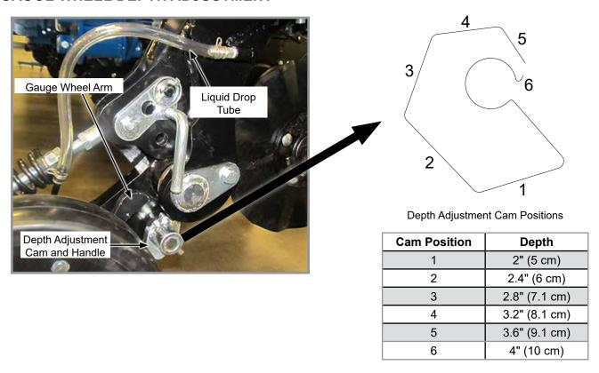
Rotate the depth adjustment cam to adjust depth of fertilizer placement into the soil.
