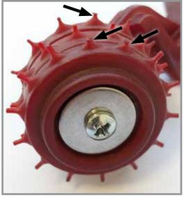
Ejector with damaged pins, indicated by arrows.
