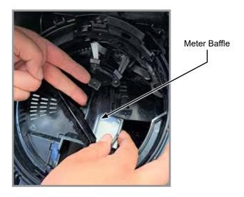
Pull the baffle door tab up (as shown below) and slide it out of the meter baffle.
