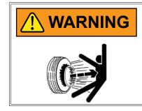
Explosive separation of rim and tire parts can cause death or serious injury. Overinflation, rim and tire servicing, improper use of rims and tires, or worn or improperly maintained tires could result in a tire explosion.
