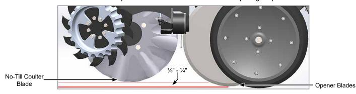
Adjust position of no-till coulter, loosen the nut and move coulter vertically to proper location.
