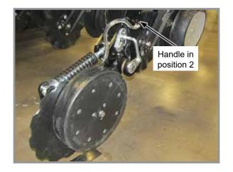
Fertilizer depth is adjustable from approximately 2" to 4" (5 to 10 cm) when planter frame is level and at proper 24" (61 cm) operating height. Soil conditions will affect fertilizer placement depth. **Do not place fertilizer any closer than 2"** (5 cm) to either side of row.
