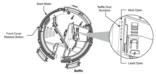
NOTE: Damaged seed or seed containing foreign material will cause plugging of seed disc orifices and require more frequent seed meter cleanout to prevent underplanting.
