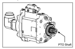
**Two-section PTO Hydraulic Pump**
