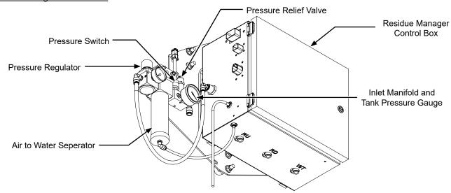
Residue Manger Control Box - Contains valves that control air pressure delivered to 3 circuits on planter.
