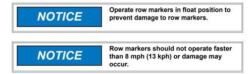
Operate row markers with Blue Vantage control or tractor's hydraulic control. After markers are lowered to ground, move hydraulic control to operate markers in float position. Marker speed is controlled with flow control valves located in planter left hand wing block. One valve controls raise speed and other valve controls lower speed of both markers. See <u>"See "Row Marker Speed Adjustment" on page 2-23</u> and <u>"See "Row Marker Cable Adjustment" on page 2-24</u>.
