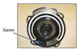
NOTE: Damaged seed or seed containing foreign material will cause plugging of seed disc orifices and require more frequent seed meter cleanout to prevent underplanting.
