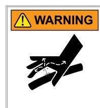
Pressurized hydraulic fluid can penetrate body tissue and result in death, serious infection, or other injuries. Fluid injected under skin must be IMMEDIATELY removed by a surgeon familiar with this type of injury. Make sure connections are tight and hoses and fittings are not damaged before applying system pressure. Leaks can be invisible. Keep away from suspected leaks. Relieve pressure before searching for leaks or performing any system maintenance.
