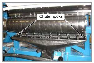
**Cleanout Chute Installed**
