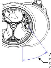
Adjust gauge wheel adjustment nut to lightly contact opener disc blade in this area for 4" to 6". Check adjustment in operating position.
