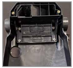
Shown with Meter Assembly Removed
