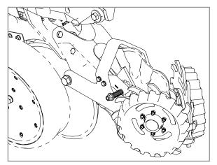
**Coulter Mounted Residue Wheels W/Treader**
