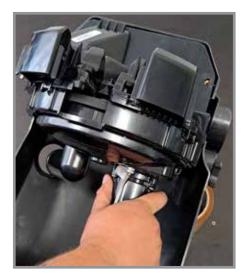
When planting canola/rapeseed is complete, remove parts installed specifically for canola/rapeseed seed disc (except for meter wall brush, it can be used with any other seed discs). Return meter back to it's original state.
