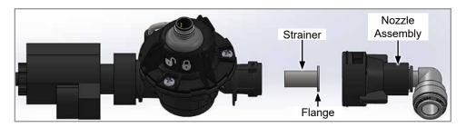
2. Pull strainer out of flow meter and clean or replace it.
