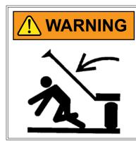
Uncontrolled marker movement can cause death or serious injury. Set marker switch to OFF and shut off tractor prior to adjustment.
