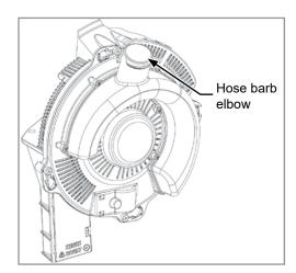
NOTE: Foreign material in seed disc orifices, such as seed chips, hulls, stems, etc., may affect seed delivery. Clean seed ensures accurate seed metering from vacuum seed meter. Remove Seed discs daily to check for buildup of foreign material in seed disc orifices.
