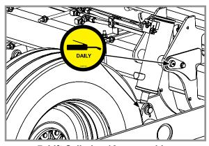
7. Lift Cylinder, 16 per machine 2 fitting per cylinder
