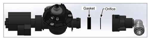
NOTE: Orifices must be installed correctly. Install orifice with the blank side towards the flow meter manifold and the stamped side facing nozzle assembly (pointing downstream toward the direction of delivery).
