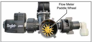
4. Once clean, place paddle wheel back onto pin inside cavity and spin the paddle wheel to ensure it is seated correctly.
