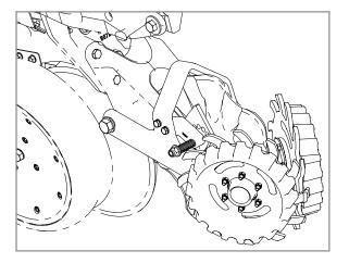
Residue wheels attach to row unit mounted coulter with two cap screws and sleeves allowing unit to free-float. A 2-position spindle bolt mounting positions wheels interlocked or staggered. Depth adjustment is made with a spring-loaded cam and pin with 8 positions in 1/16" (6 mm) increments. A high point on the cam allows wheels to be locked up.
