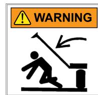
Row marker can lower at any time and could cause death or serious injury. Stay away from row markers! Install safety lockup device when not in use.
