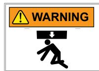
Uncontrolled movement of equipment can cause loss of control and could result in death, serious injury, or damage to property and equipment. Install all safety lockup devices before transporting equipment.
