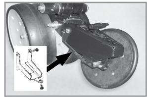
Closing Wheel Shield (closing wheel removed)
