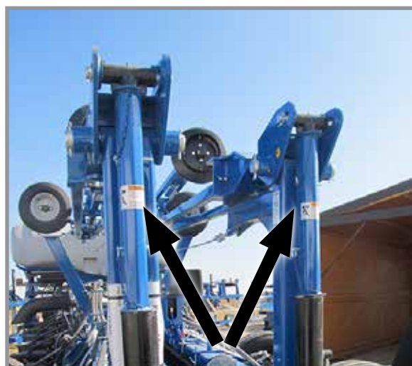
Row Marker Safety Lockup Installed
