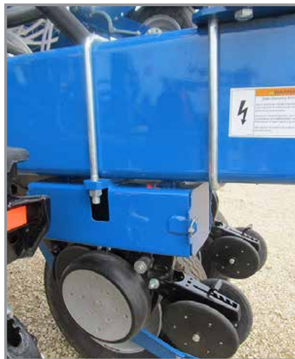
Cylinder lockup storage tube
