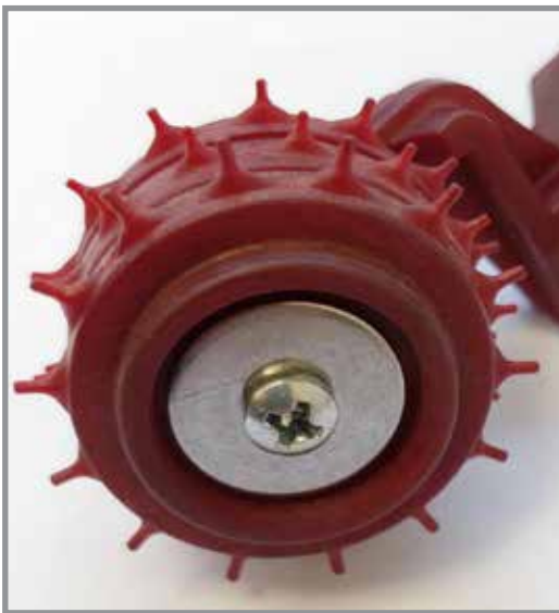
Ejector with intact pins
