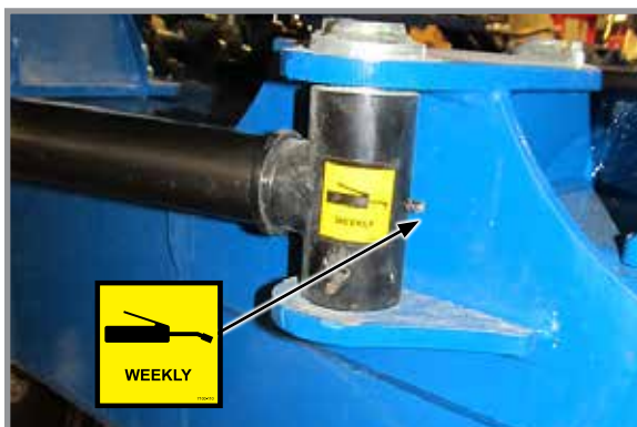
3. Fold cylinders, 2 per machine 2 fittings per cylinder (one each end)
