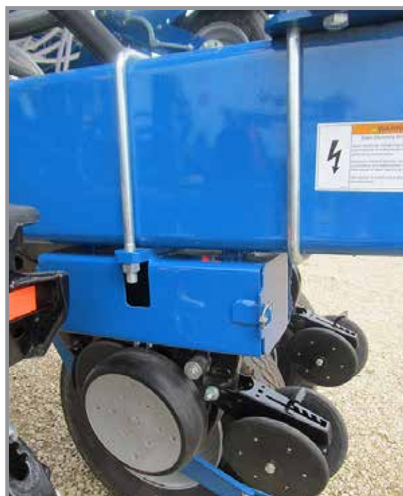
Cylinder lockup storage tube
