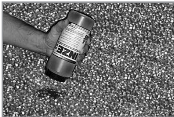
Adding graphite bulk fill hopper
