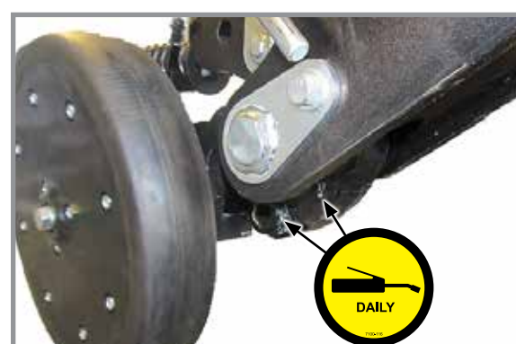
Grease to purge - 2 fittings
