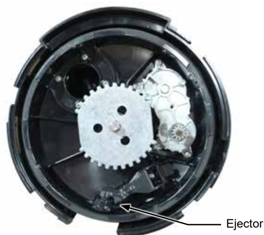
Seed Meter With Back Cover Removed
