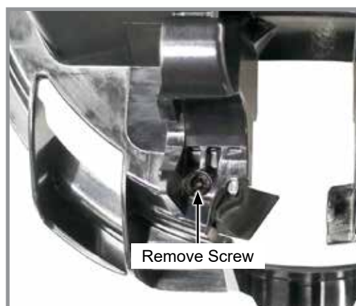
Style B: Remove one screw.
