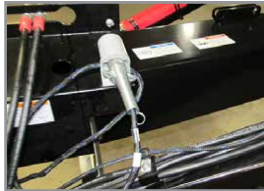
7-pin Electrical Connector Storage
