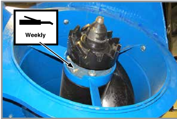
Vertical Auger Center Bearing - 1 fitting
