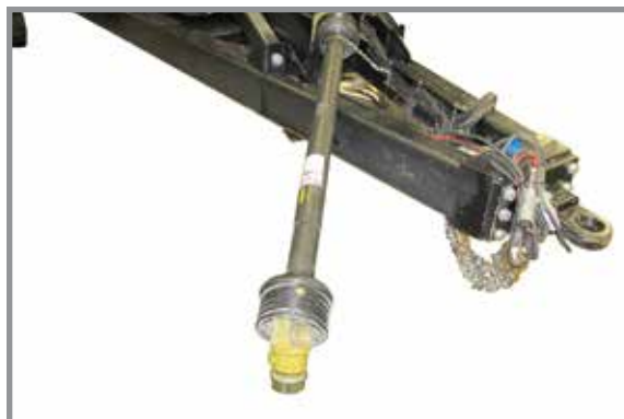
PTO shaft positioned for tractor hookup
