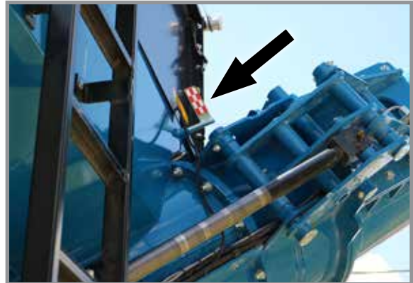
Flow Gate Position Indicator
