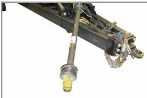
PTO shaft positioned for tractor hookup
