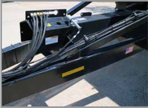
Hydraulic Hose Storage
