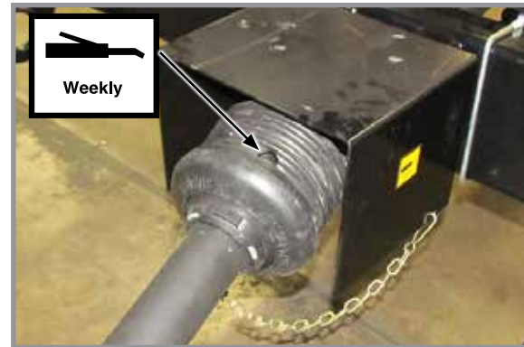
Intermediate Drive Line, Center - 1 fitting
