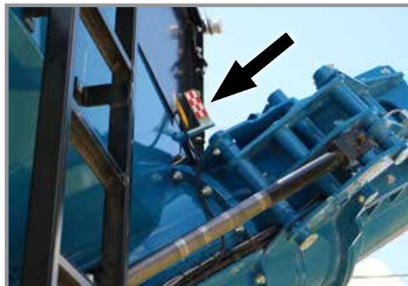
Flow Gate Position Indicator
