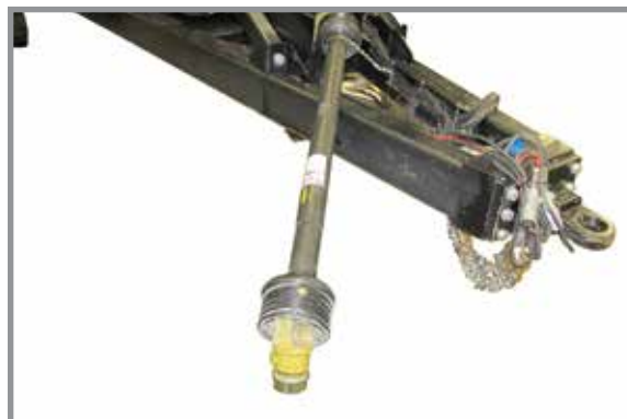
PTO shaft positioned for tractor hookup
