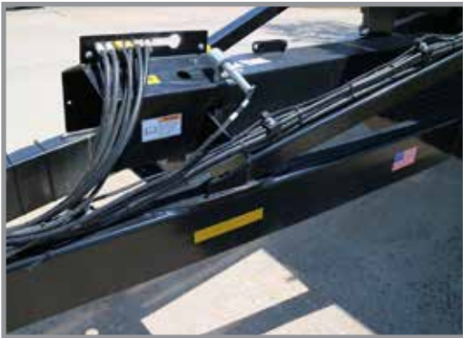
Hydraulic Hose Storage
