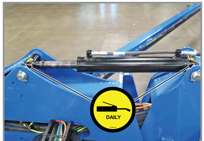
11. Wing Down Pressure Cylinders, 2 per machine 2 fittings per cylinder
