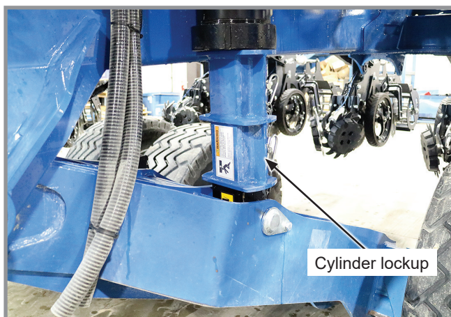
Transport axle cylinder lockup installed
