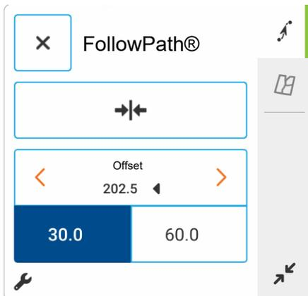
b. The offset number shown on screen is the distance from the right side of the current pass
