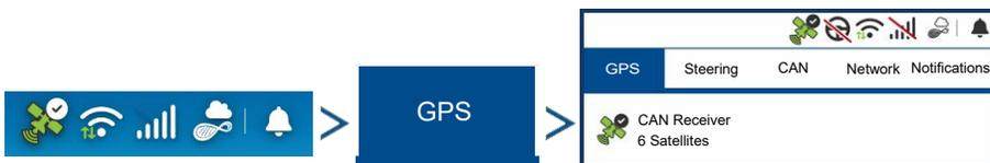
Information specific to a connected receiver is available by selecting an available unit under the GPS tab in diagnostics.
