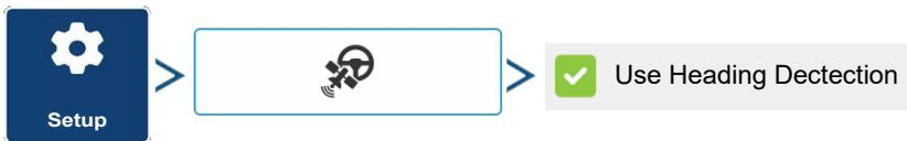
With Heading Detection disabled, the icon will always follow the GPS heading. When using a Harvest configuration, Heading Detection is automatically disabled regardless of the state of the enable/disable button.
