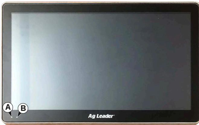
A. **Light sensitivity sensor**—Used to automatically dim the display during night-time or low-light situations.
