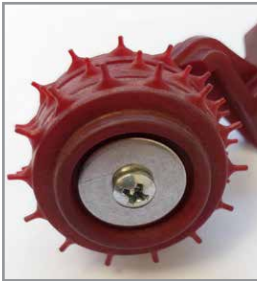
Ejector with intact pins
